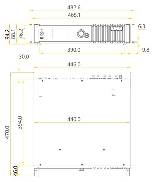
Tolerance: ±0.3 Unit: mm
